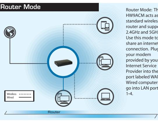
Router Mode: The HW9ACM acts as a standard wireless router and supports 2.4GHz and 5GHz AC. Use this mode to share an internet connection. Plug provided by your Provider into the port labeled WAN. Wired computers can go into LAN ports
