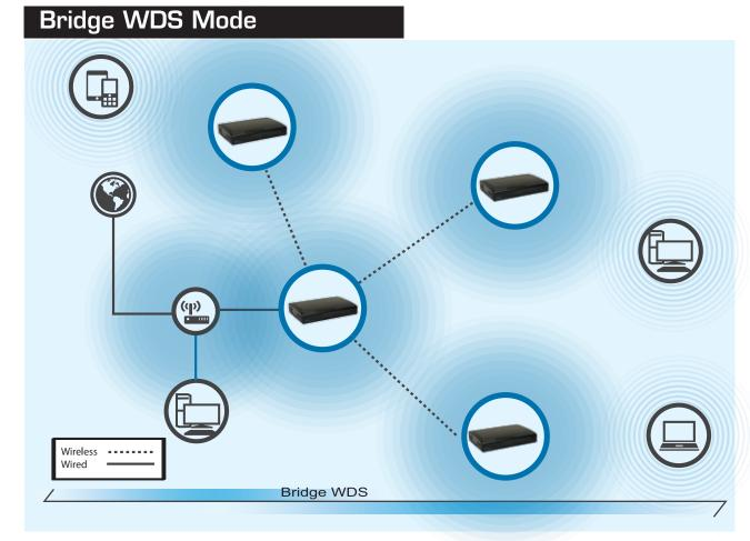
Bridge WDS Mode: The HW9ACM allows you to connect up to 4 HW9ACM's wirelessly to each other to expand the scope of your network. In this mode, the HW9ACM will transmit a wireless signal. Be sure to use the same SSID, channel and security for each. The first HW9ACM must be connected to the primary network via LAN port 1-4 and the others can be standalone.
