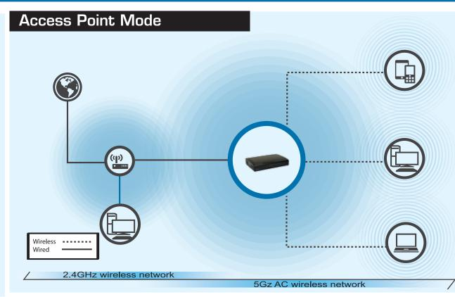
**Access Point** Mode: The HW9ACM acts as a standard wireless access point. It can upgrade your existing 2.4GHz WiFi network to a 5GHz AC or expand it, giving it greater coverage. After setup, be sure to hook the HW9ACM to your network via LAN ports 1-4.
