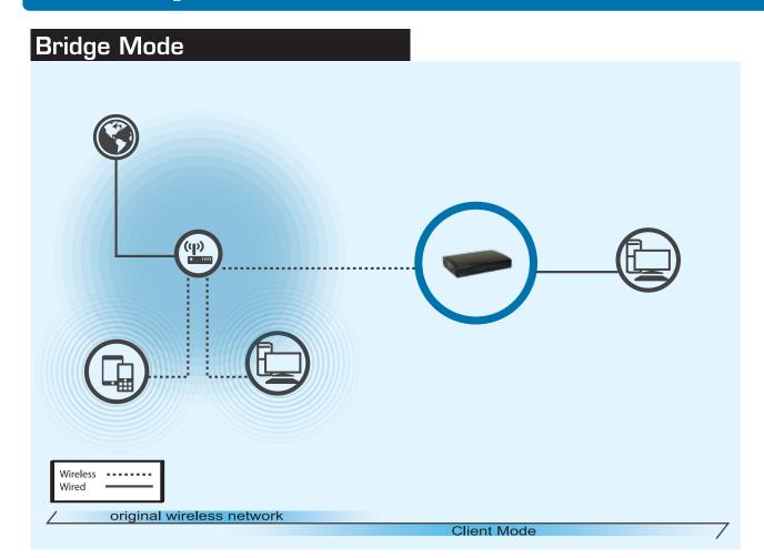
Bridge Mode: The HW9ACM allows you to connect wired devices wirelessly to an existing wireless router or access point. Non-wireless devices can network wirelessly with your Wireless Network. In this mode, the HW9ACM does not broadcast any wireless signal. After setup, be sure to hook it up to client computers/devices via LAN ports 1-4.
