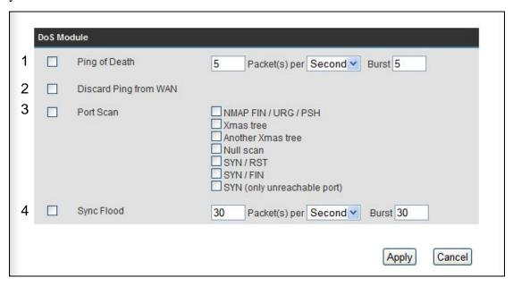
Ping of Death (1): Set the threshold of when this DoS prevention mechanism will be activated. Please check the box of Ping of Death, and input the
