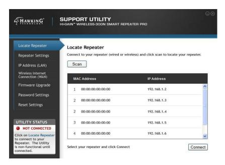
Note: before making any configurations on the Utility, you MUST be connected to a Repeater. The status of the Utility and Repeater connection is displayed on the bottom left corner.
