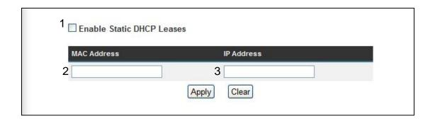
Enable Static Check this box to enable this function,
