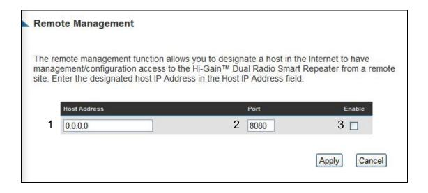
Host Address (1): Input the IP address of the remote host you wish to initiate a management access.
