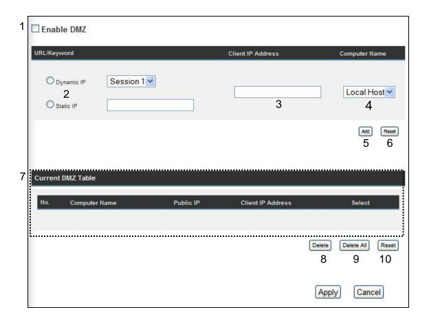
Enable DMZ (1): Check this box to enable DMZ function, uncheck this box to disable DMZ function.
