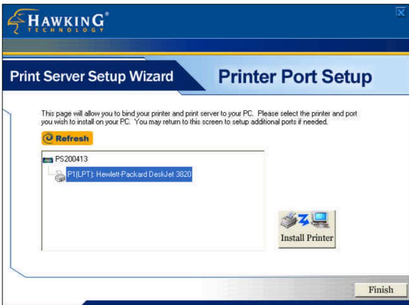
Please select the appropriate printer you wish to connect to the print server and press the “**Install Printer**” button.
