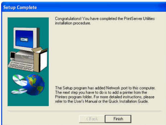
9. Once the Setup Wizard is activated, it will make sure you have the necessary components to proceed with installation. Please make sure you have connected your print server to your network via an Ethernet connection, powered up your printer and print server, and have connected the print server to your printer.
