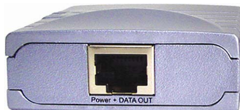
Figure 4. The Injector's Power + Data-Out port
