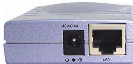
Figure 3. The Injector's Data-In and Power-In ports
