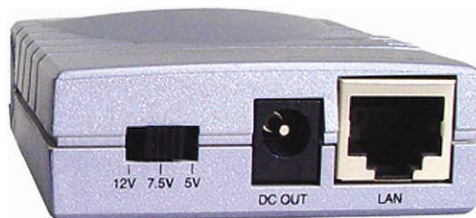
Figure 6. The Splitter's Data-Out port, Power Out port, and DIP Switch
