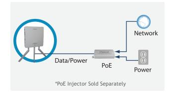
By combining your power and data connections into a single cable, PoE can simplify the setup. This gives you flexibility to install the device in any location, even out of the way locations with few power outlets.
