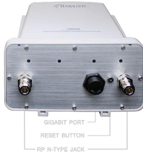
Hawking Technology's HOD45B outdoor multifunction wireless device offers the best solution for both range and data intensive network environments. It is designed with multiple solutions in one high performance, weather-proof, outdoor unit. The HOD45B features a Power-over-Ethernet connection and comes with wall and pole mounting kits. Built-in 2.4GHz and 5.0GHz radios simultaneously support the IEEE 802.11a/b/g/n wireless network standards for streaming movies and other online applications.
