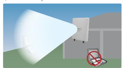
Once you have mounted and connected your Outdoor Wireless-AC 12dBi Directional Antenna, be sure to note the signal pattern of the antenna. As indicated by the diagram above, the directional antenna does not give off signal directly below or directly behind the product. Make sure your devices are within the signal pattern shown above to experience superior range and quality with your HOA12DP. Adjust the antenna as needed.
