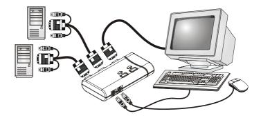
**DO NOT TRY** to connect the KVM Switch to the computers while the computers are still in powered-on states. Otherwise, the computer will have difficulty recognizing your shared keyboard and mouse.
