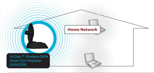
The Smart Repeater will not work without a signal it can repeat. Make sure to place the HAW2DR within the receiving range, usually around 150-200ft\* from the Wi-Fi Router / Access Point. Line of sight is recommended for the best Wi-Fi reception.
